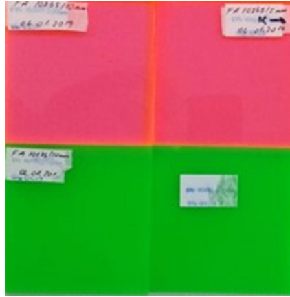
Figure 2. 4 acrylic samples having two different thicknesses and colors.
